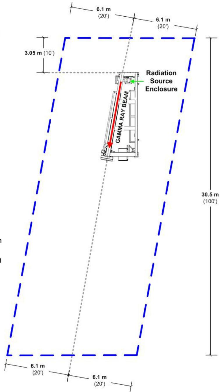
**Figure 1: Radiation Controlled Area (without Shield Material)**
