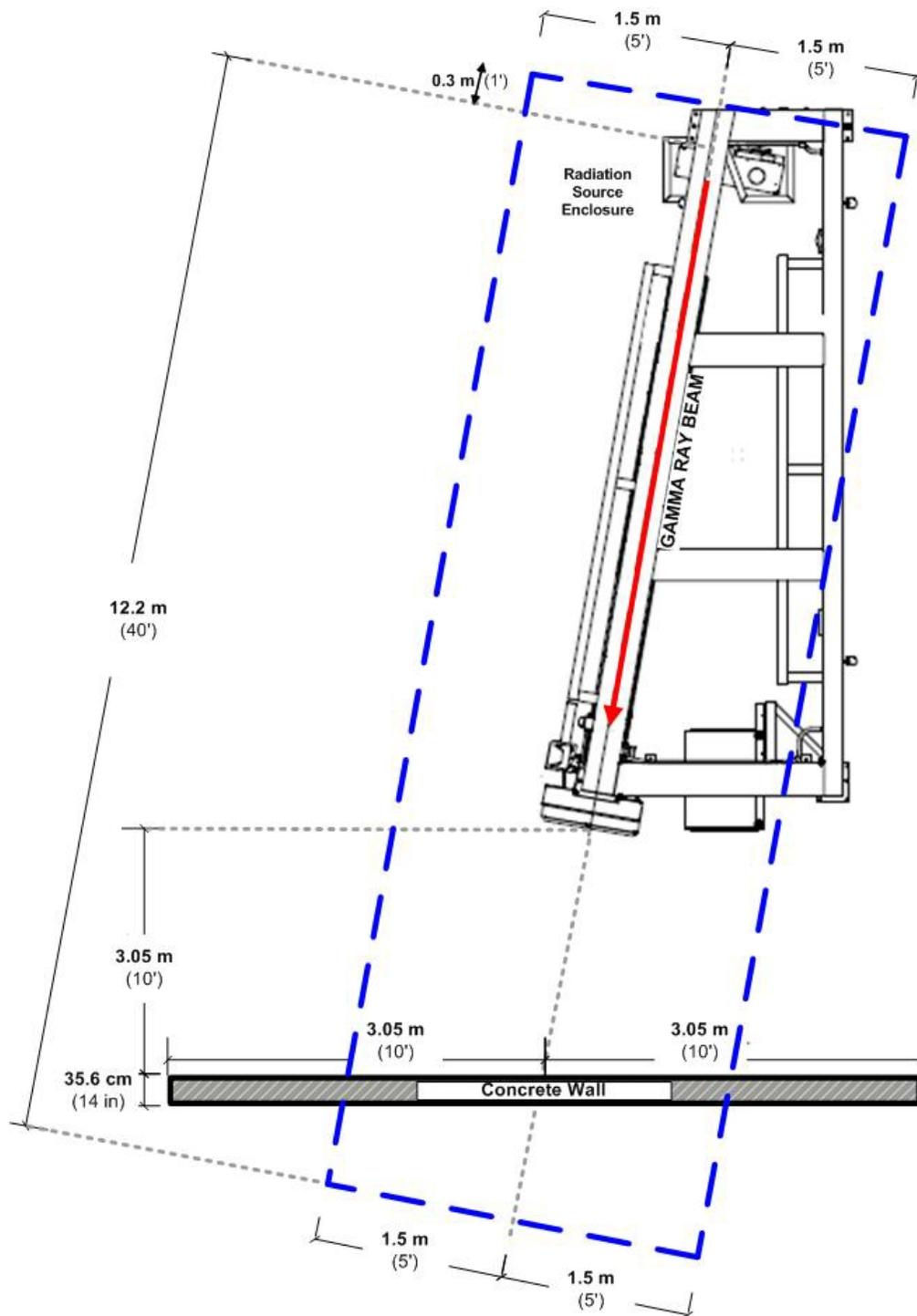
**Figure 4: Radiation Exclusion Zone with Shield Material**
