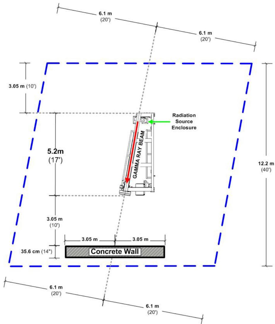
Figure 2: Radiation Controlled Area with Shield Material
