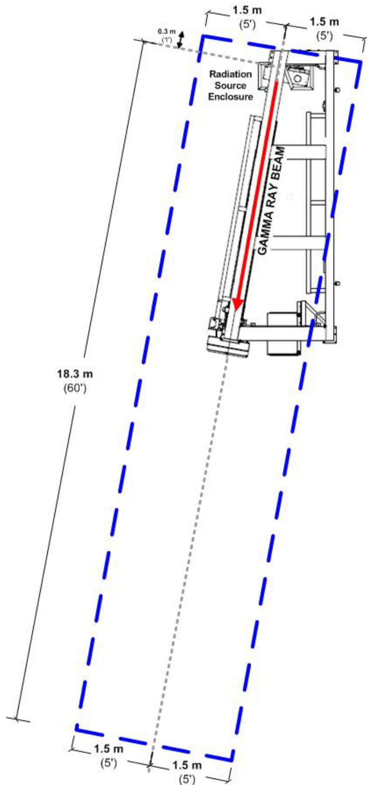
**Figure 3: Radiation Exclusion Zone (without Shield Material)**
