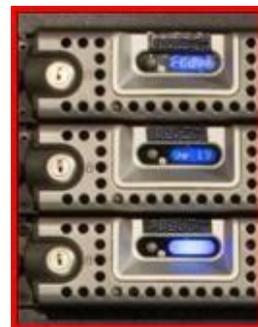
**Figure 5: Key-Locks on the Server Cabinet and on each Server**
