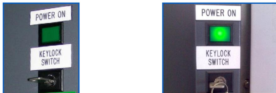
Figure 6: Green POWER ON Button and Key-Lock Switch on the Scanner
